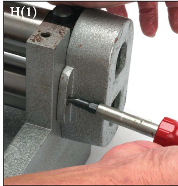
H)-1,2 Remove the Side Gear Cover that is secured with two screws.
