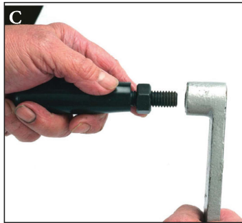
C) Screw the small handgrip handle into the large handle.
