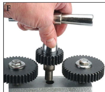
F) Once you have the top gears balanced install the T-top roller adjuster
