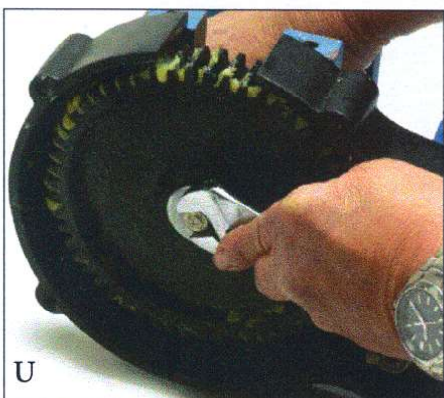
U) Remove the bolt that holds the large reduction gear to the mill.
