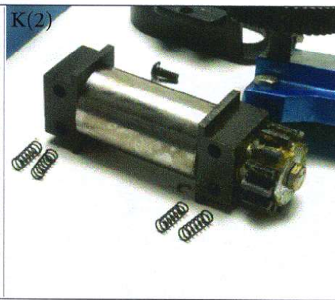
K-1, 2) Remove top roller-Note: Be careful with the springs between upper and lower rollers, they provide tension and are very important. In order to prevent loss, put aside in a safe spot until reinstalling them.
