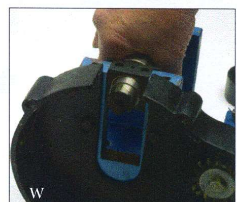
W) You can now access the lower roller and remove it from the mill.
