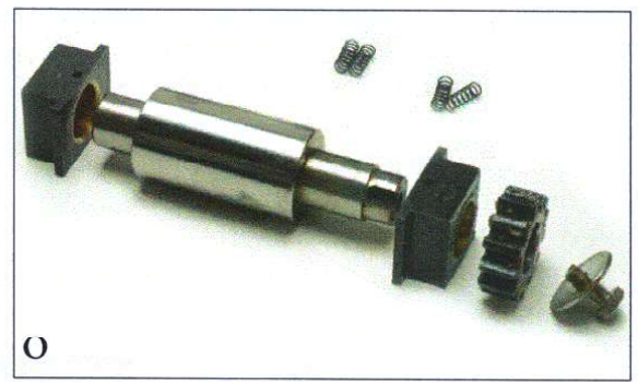
O) You have now disassembled the upper roll.
