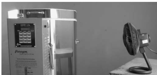
Hot weather pointer: Blow a gentle stream of air through the control panel of the kiln to reduce the temperature of the controller circuit board.
