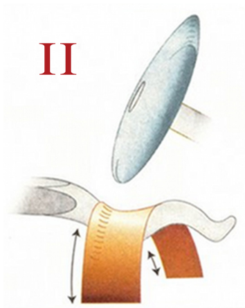
Diagram I3 Return the furrowed piece to the sinusoid, so the point of contact between the metal and stake will be at the base of the first two furrows.
