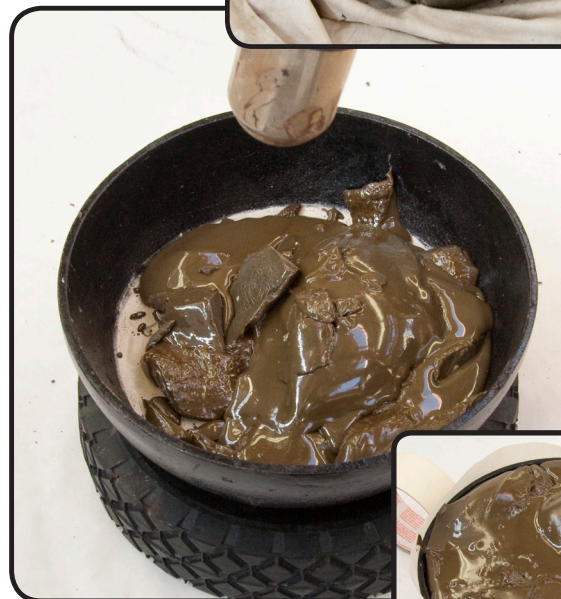
Melting the pitch with a hot-air gun, and finishing a bowl with a tape collar.
