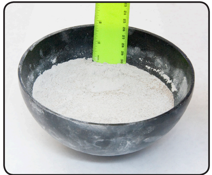
8" bowl with .9 kilos of cement mix leaves 1.75" of depth.
