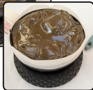
Melting the pitch with a hot-air gun, and finishing a bowl with a tape collar.
