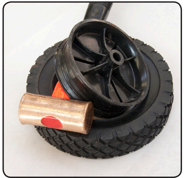
A hardware store wagon wheel with the hub knocked out makes a fine base ring for about $5
